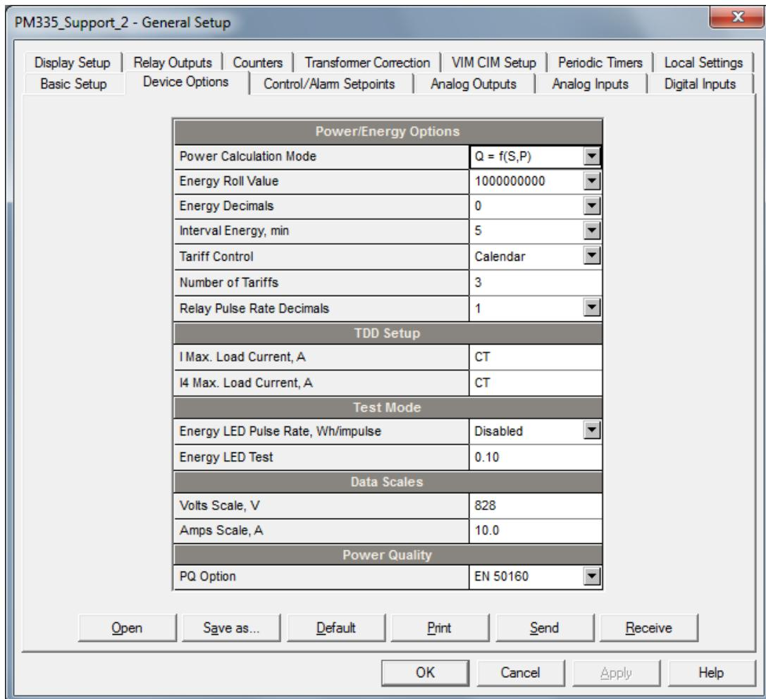
The following device settings affect IEEE 519 evaluation and should be checked prior to running the IEEE 519 PQ recorder.
