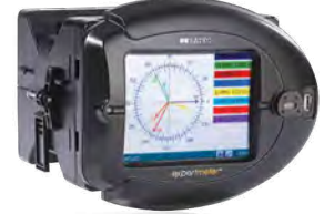
PHASOR MEASUREMENT UNIT
