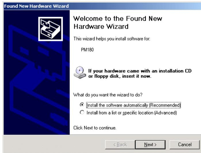
2. Insert the PAS Installation CD into the CD ROM Drive, select “Install the software automatically”, and then click “Next”. Windows XP finds and installs the required driver automatically.
