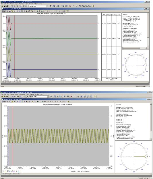
You can open all five views together to analyze different properties of the waveform like a wave shape, waveform disturbance, unbalance, or spectrum. When you move to another waveform record, all views are updated simultaneously to reflect the changes.
