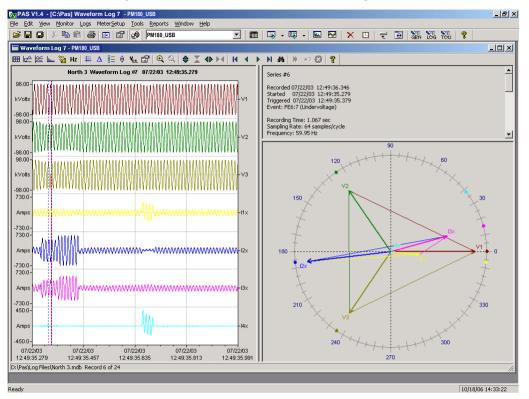
To change the reference channel, click on the waveform window with the right mouse button, select "Options...", click on the "Phasor" tab, check the channel you want to make a reference channel, and then click "OK".
