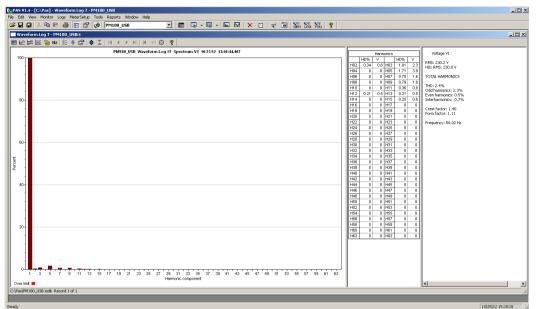
The order of the highest displayed harmonic component is equal to the half sampling rate at which the waveforms are sampled minus one. If the waveform was sampled at a rate of 256 samples per cycle, 63 harmonics are available. With 32 samples per cycle, only 15 harmonics are calculated, while others will be zeros.
