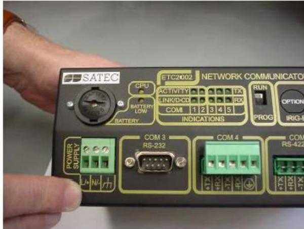
Figure 7-1 Battery Housing Location of the Panel
