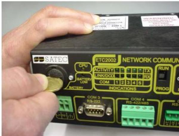
Figure 7-2 Battery Housing Cover Removal
