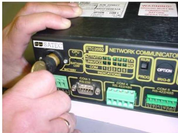
Figure 7-4 Insertion of New Battery
