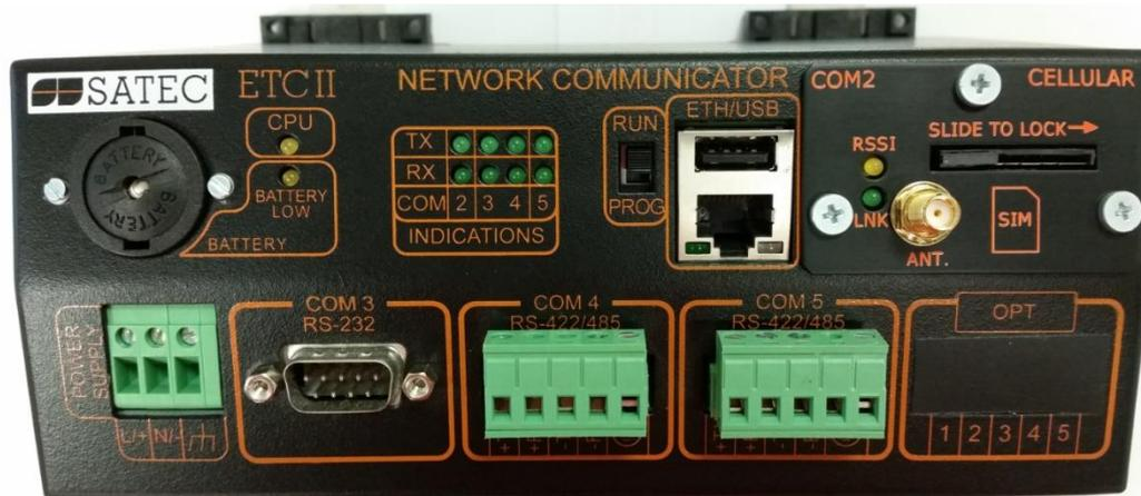
**Figure 3-1 Indicator LEDs**
