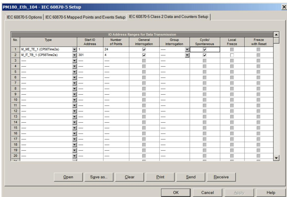
2. Select object type and specify ranges of points to be included into interrogation responses or/and cyclic/spontaneous data transmission. Only mapped point addresses (see Section 6.2) and general object addresses listed in Section 3.2 can be used for interrogation and cyclic/spontaneous transmission. See Section 3.2 for compatible object types.
