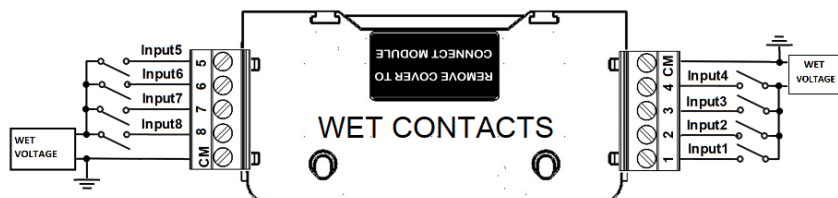
Figure 2-22 8 DI - Digital Input Connection – Wet contact model
