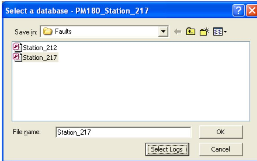
4. Click "Select Logs" and check the fault log box, and the boxes for the data and waveform log files you selected for recording fault waveforms and distance calculations results in the Fault Recorder setup.
