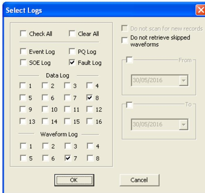
To view the recorded fault distance data, select Open... in the File menu, point to the database with the uploaded data and double click on the data log table on the right pane.
