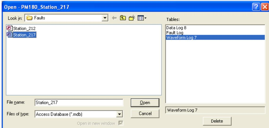
3. Select a fault waveform for which you want to calculate the fault distance. See "Viewing Waveforms" in the PM180 Operation Manual for more information on viewing options.
