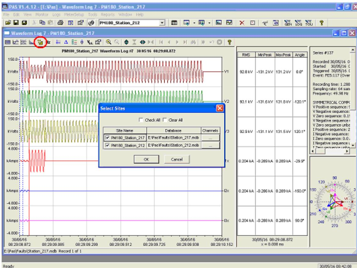
5. Check the two-sided waveforms to be used for distance calculations. You can also select the waveform channels you want to view for each site by clicking the button on the right to the site. An example of two synchronized waveforms is shown in the picture below.
