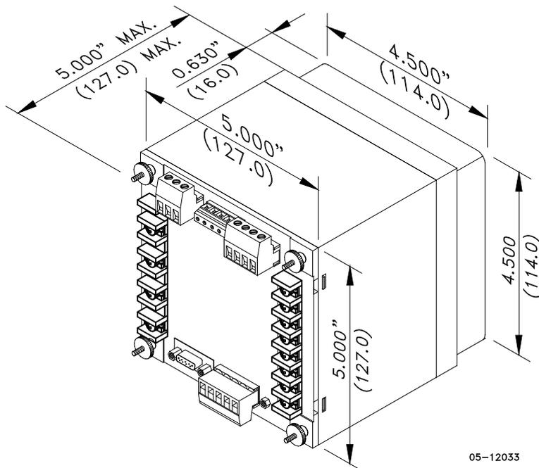
**Figure 1: Instrument Dimensions**
