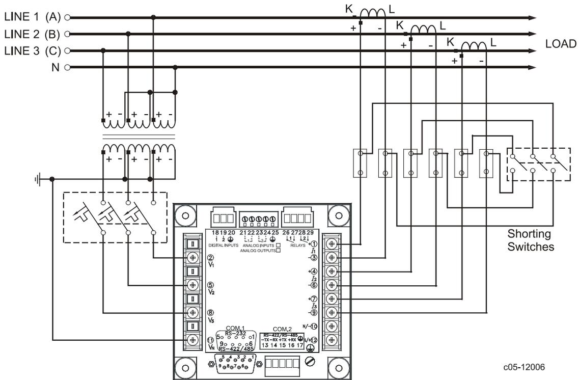
**Figure 6: Typical Installation 1**
